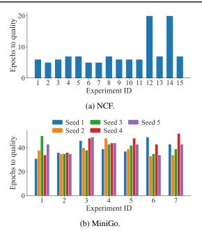
Figure 1. Training epochs to reach the target quality for the MLPerf v0.5 NCF (a) and MiniGo (b) benchmarks. Each experiment uses identical hyperparameters except for the random seed. For MiniGo, we observed considerable variability across runs even when fixing the random seed (same color).
