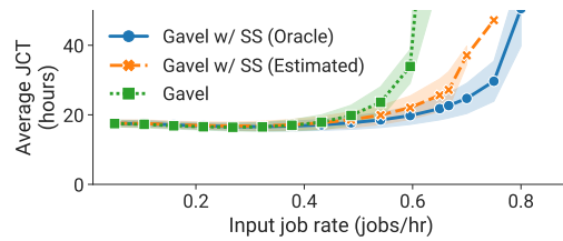
Figure 16: Comparison of SS-aware LAS policy with estimated throughputs, compared to the SS-aware with oracle throughputs and LAS without space sharing on a heterogeneous 12-GPU cluster.
